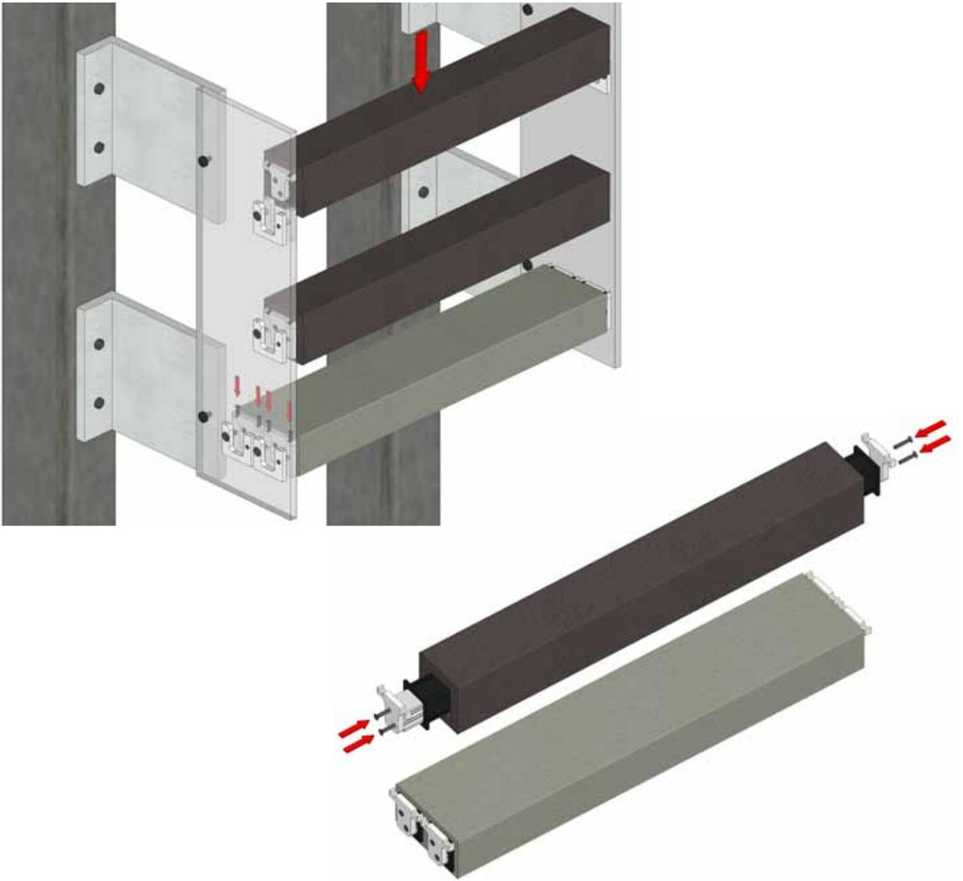
Construct a baguette/louver assembly with aluminum spline and gaskets as outlined on page 6. Attach the “T” part of the bracket assembly to the spline at each end of the baguette/louver assembly using the specified fastener or pinning method.
