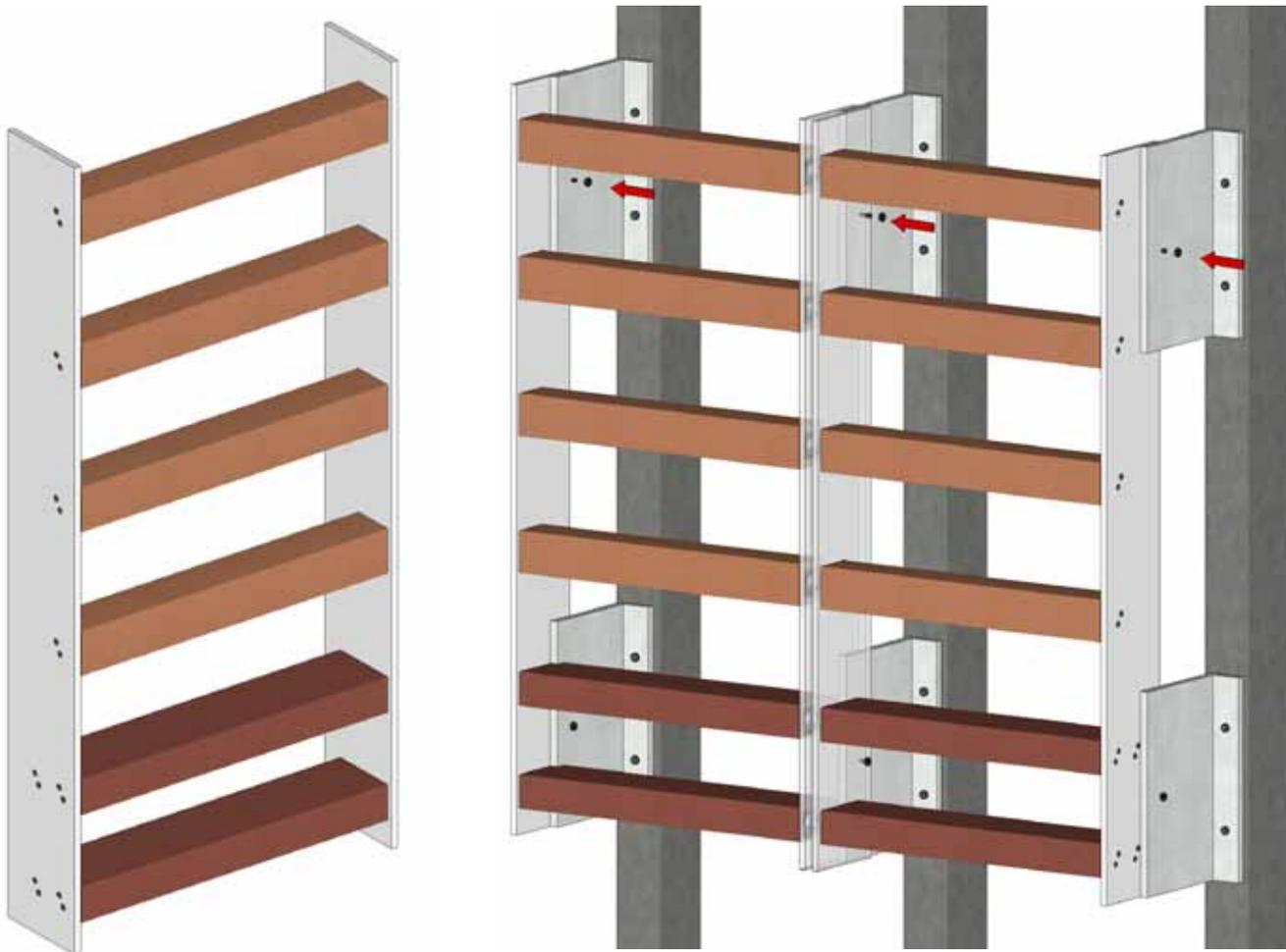
Once a complete baguette/louver arrangement is installed within a pair of aluminum fin plates, the entire unitized assembly can be moved into place.
